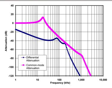
Figure 1: Simulation of calculated common-mode and differential-mode current attenuation. The plots show the ratio of the measured current in a  $50\Omega$  LISN sensing port connected to pins 1 or 3 to the noise current injected into pins 4 and 6. See Figs. 2 & 3.
