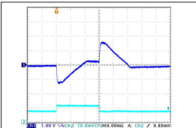
Figure 5: Output voltage response to step-change in load current (50%-75%-50% of I<sub>out(max)</sub>; dI/dt = 0.1A/μs. Load cap: 100μF electrolytic cap and 1μF ceramic cap. Ch 1: V<sub>out</sub>, Ch 2: I<sub>out</sub> (5 A/div).
