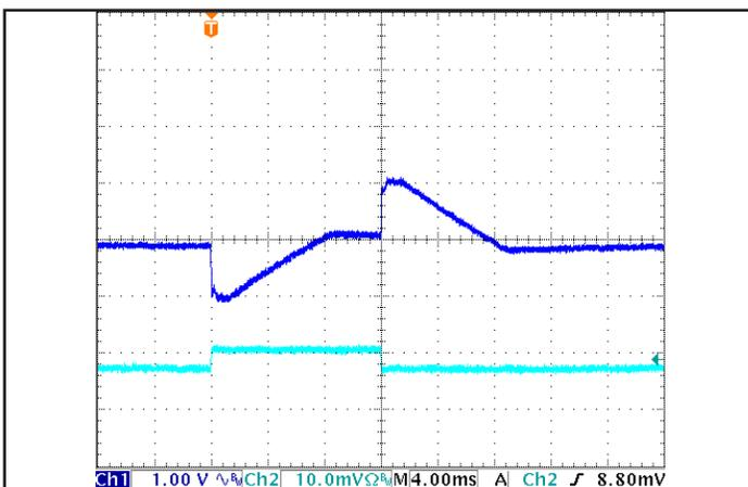
Figure 5: Output voltage response to step-change in load current (50%-75%-50% of I<sub>out</sub>(max); dI/dt = 0.1A/μs. Load cap: 100μF electrolytic cap and 1μF ceramic cap. Ch 1: V<sub>out</sub>, Ch 2: I<sub>out</sub> (10 A/div).
