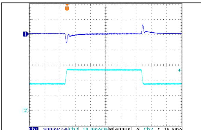
Figure 5: Output voltage response to step-change in load current (66 %–100 %–66 % of Iout(max);  $dI/dt = 0.1 \text{ A}/\mu\text{s}$ ). Load cap: 1  $\mu\text{F}$  ceramic and 15  $\mu\text{F}$  tantalum capacitor. Ch 1: Vout (500 mV/div), Ch 2: Iout (5 A/div).
