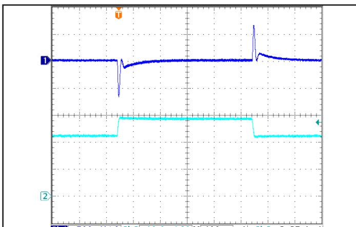
Figure 5: Output voltage response to step-change in load current (66 %–100 %–66 % of Iout(max);  $dI/dt = 0.1 A/\mu s$ ). Load cap: 1  $\mu F$  ceramic and 15  $\mu F$  tantalum capacitors. Ch 1: Vout (500 mV/div), Ch 2: Iout (2 A/div).
