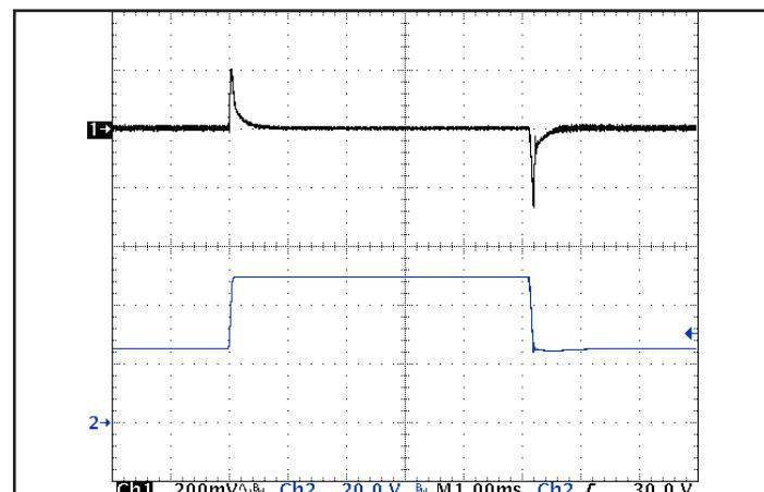
Figure 6: Output voltage response to step-change in input voltage (500 V/ms). Load cap: 100  $\mu\text{F}$ , electrolytic output capacitance. Ch 1: Vout (200 mV/div), Ch 2: Vin (20 V/div).
