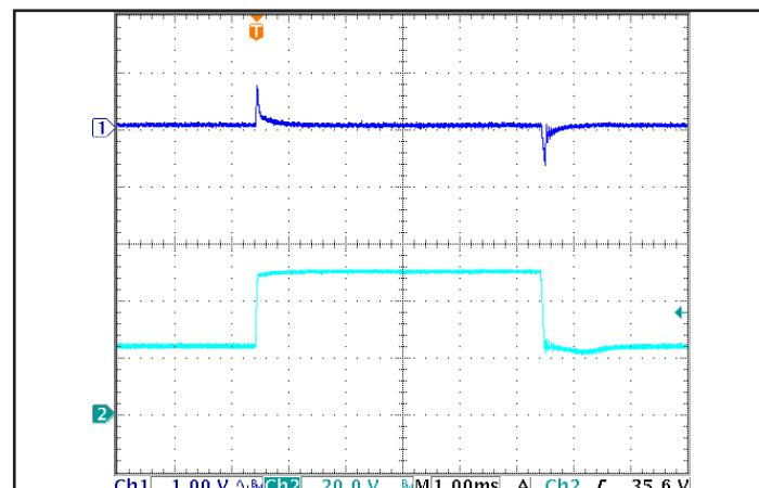
Figure 6: Output voltage response to step-change in input voltage (500 V/ms). Load cap: 100  $\mu\text{F}$  electrolytic output capacitance. Ch 1: Vout (1 V/div), Ch 2: Vin (20 V/div).
