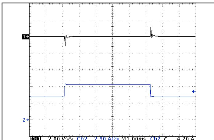
Figure 5: Output voltage response to step-change in load current (66 %–100 %–66 % of Iout(max);  $dI/dt = 0.1 \text{ A}/\mu\text{s}$ ). Load cap: 1  $\mu\text{F}$  ceramic capacitor. Ch 1: Vout (2 V/div), Ch 2: Iout (2.5 A/div).
