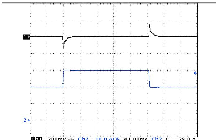
Figure 5: Output voltage response to step-change in load current (66 %–100 %–66 % of Iout(max);  $dI/dt = 0.1 \text{ A}/\mu\text{s}$ ). Load cap: 1  $\mu\text{F}$  ceramic and 15  $\mu\text{F}$  tantalum capacitors. Ch 1: Vout (200 mV/div), Ch 2: Iout (10 A/div).
