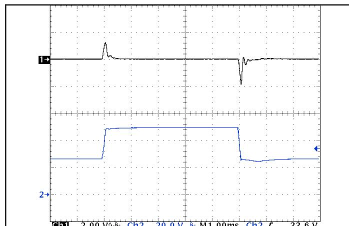
Figure 6: Output voltage response to step-change in input voltage (500 V/ms). Load cap: 100  $\mu\text{F}$ , electrolytic output capacitance. Ch 1: Vout (2 V/div), Ch 2: Vin (20 V/div).
