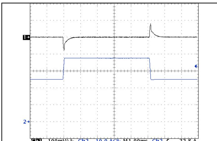
Figure 5: Output voltage response to step-change in load current (66 %–100 %–66 % of  $I_{out(max)}$ ;  $dI/dt = 0.2 A/\mu s$ ). Load cap: 1  $\mu F$  ceramic and 15  $\mu F$  tantalum capacitors. Ch 1:  $V_{out}$  (100 mV/div), Ch 2:  $I_{out}$  (10 A/div).
