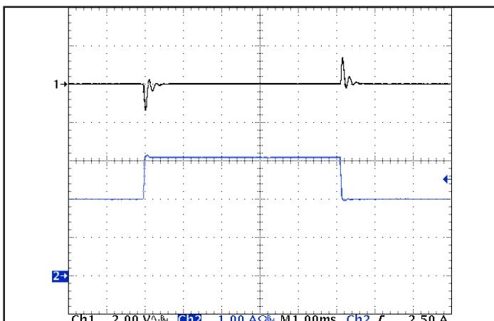
Figure 5: Output voltage response to step-change in load current (66 %–100 %–66 % of Iout(max);  $dI/dt = 0.05 \text{ A}/\mu\text{s}$ ). Load cap: 1  $\mu\text{F}$  ceramic capacitor. Ch 1: Vout (2 V/div), Ch 2: Iout (1 A/div).
