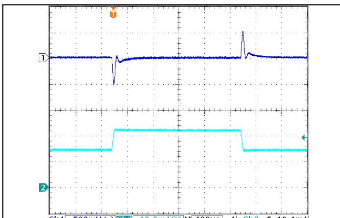
Figure 5: Output voltage response to step-change in load current (66 %–100 %–66 % of Iout(max);  $dI/dt = 0.1 A/\mu s$ ). Load cap: 1  $\mu F$  ceramic and 15  $\mu F$  tantalum capacitors. Ch 1: Vout (500 mV/div), Ch 2: Iout (5 A/div).
