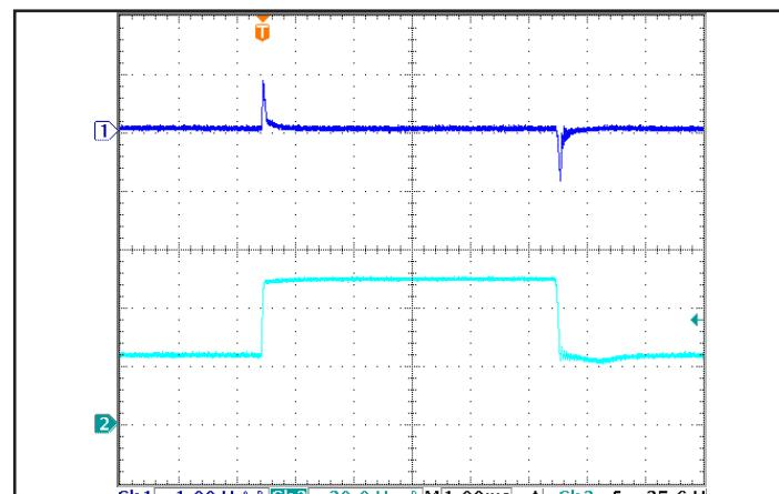
Figure 6: Output voltage response to step-change in input voltage (500 V/ms). Load cap: 100  $\mu F$  electrolytic output capacitance. Ch 1: Vout (1 V/div), Ch 2: Vin (20 V/div).
