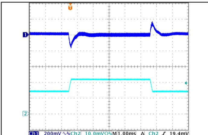
Figure 5: Output Voltage Response to Step-Change in Load Current (50%-75%-50% of I<sub>out</sub>(max); dI/dt = 0.2A/μs). Load cap: 15μF tantalum cap and 1μF ceramic cap. Ch 1: V<sub>out</sub>, Ch 2: I<sub>out</sub> (20A/div).
