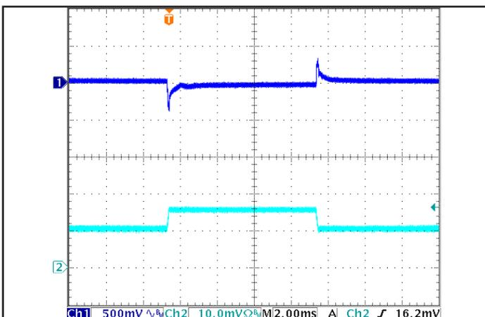
Figure 5: Output Voltage Response to Step-Change in Load Current (50%-75%-50% of I<sub>out</sub>(max)); dI/dt = 0.1A/μs. Load cap: 15μF tantalum cap and 1μF ceramic cap. Ch 1: V<sub>out</sub>, Ch 2: I<sub>out</sub> (20 A/div).
