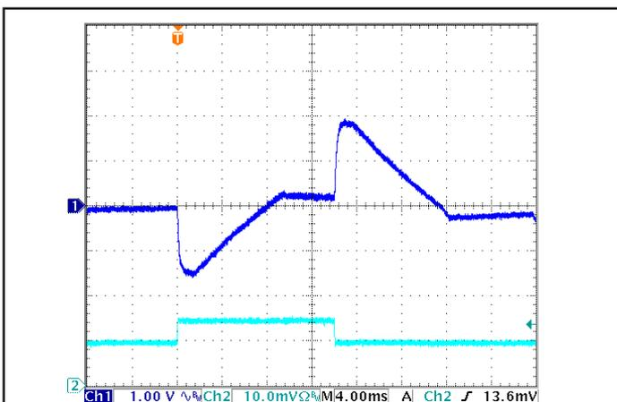
Figure 5: Output Voltage Response to Step-Change in Load Current (50%-75%-50% of I<sub>out</sub>(max)); dI/dt = 0.1A/μs. Load cap: 100μF electrolytic cap and 1μF ceramic cap. Ch 1: V<sub>out</sub>, Ch 2: I<sub>out</sub> (5 A/div).
