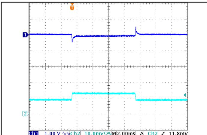
Figure 5: Output Voltage Response to Step-Change in Load Current (50%-75%-50% of I<sub>out</sub>(max)); dI/dt = 0.1A/μs. Load cap: 15μF tantalum cap and 1μF ceramic cap. Ch 1: V<sub>out</sub>, Ch 2: I<sub>out</sub> (20 A/div).
