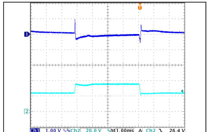
Figure 6: Output Voltage Response to Step-Change in Input Voltage (250 V/ms), at Max. load current. Load cap: 100μF electrolytic cap and 1μF ceramic cap. Ch 1: V<sub>out</sub>, Ch 2: V<sub>in</sub>.
