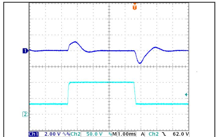
Figure 6: Output voltage response to step-change in input voltage (nominal to maximum), at full load current. Load cap: 1 μF ceramic cap. Ch 1: V<sub>out</sub>, Ch 2: V<sub>in</sub>.
