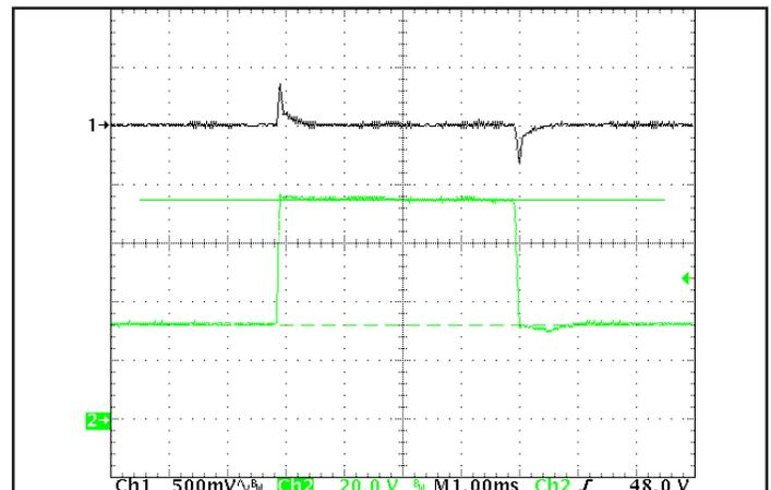
Figure 6: Output voltage response to step-change in input voltage (nominal to maximum), at full load current. Load cap: 15 μF tantalum capacitor and 1 μF ceramic cap. Ch 1: V<sub>out</sub>, Ch 2: V<sub>in</sub>.
