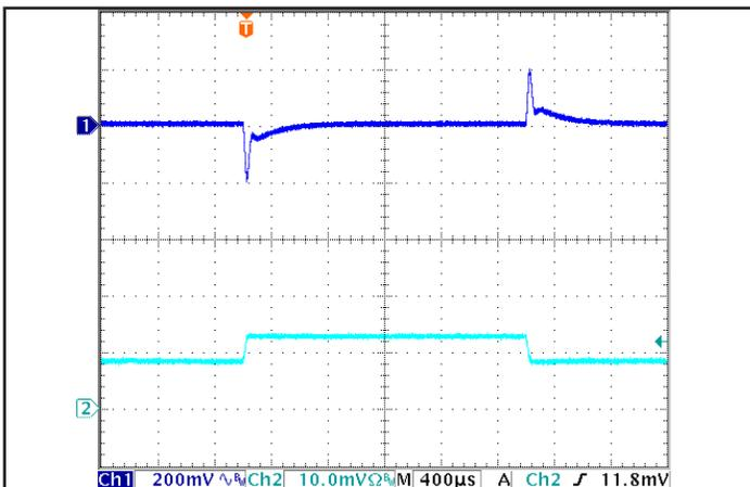
Figure 5: Output voltage response to step-change in load current (50% -75% -50% of I<sub>out</sub>(max); dI/dt = 0.6 A/μs). Load cap: 15 μF tantalum cap and 1 μF ceramic cap. Ch 1: V<sub>out</sub>, Ch 2: I<sub>out</sub> (10 A/div).
