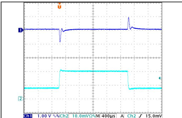
Figure 5: Output voltage response to step-change in load current (50% -75% -50% of I<sub>out</sub>(max); dI/dt = 0.6 A/μs). Load cap: 15 μF tantalum cap and 1 μF ceramic cap. Ch 1: V<sub>out</sub>, Ch 2: I<sub>out</sub> (2 A/div).
