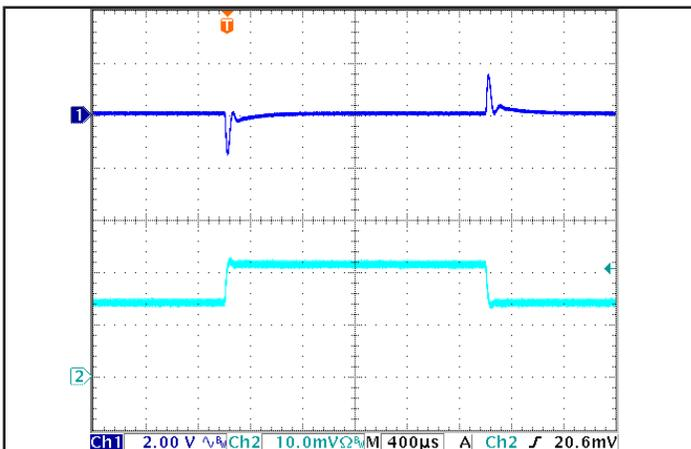
Figure 5: Output voltage response to step-change in load current (50% -75% -50% of  $I_{out(max)}$ ;  $dI/dt = 0.6 A/\mu s$ ). Load cap: 1  $\mu F$  ceramic cap. Ch 1:  $V_{out}$ , Ch 2:  $I_{out}$  (1 A/div).
