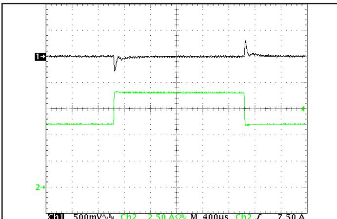
Figure 5: Output voltage response to step-change in load current (50% -75% -50% of I<sub>out</sub>(max); dI/dt = 0.6 A/μs). Load cap: 15 μF tantalum cap and 1 μF ceramic cap. Ch 1: V<sub>out</sub>, Ch 2: I<sub>out</sub>.
