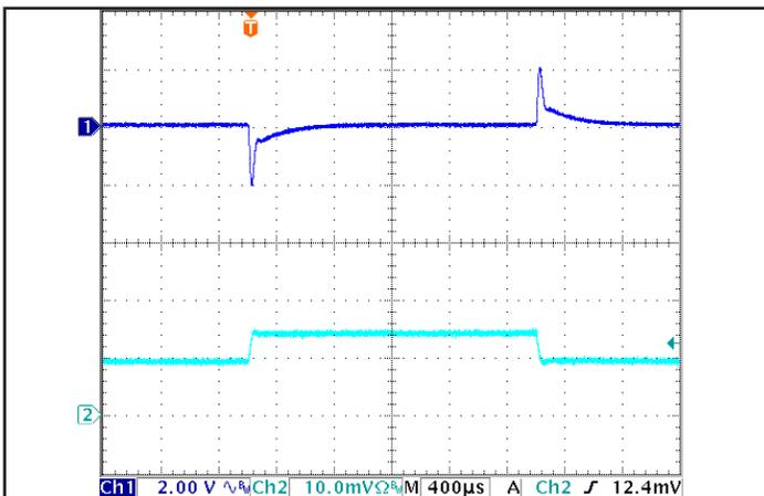
Figure 5: Output voltage response to step-change in load current (50% -75% -50% of I<sub>out</sub>(max); dI/dt = 0.6 A/μs). Load cap: 1 μF ceramic cap. Ch 1: V<sub>out</sub>, Ch 2: I<sub>out</sub> (1 A/div).
