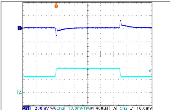
Figure 5: Output voltage response to step-change in load current (50% -75% -50% of  $I_{out(max)}$ ;  $dI/dt = 0.6 A/\mu s$ ). Load cap: 15  $\mu F$  tantalum cap and 1  $\mu F$  ceramic cap. Ch 1:  $V_{out}$ , Ch 2:  $I_{out}$  (10 A/div).
