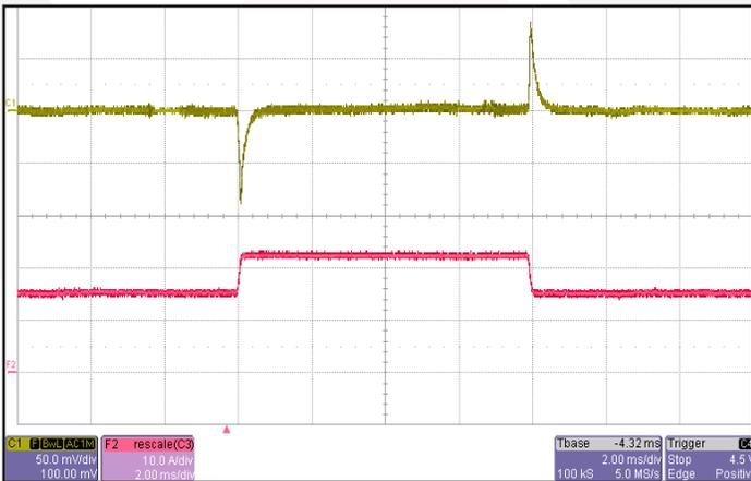
**Figure 11:** Output voltage response to step-change in load current (50%-75%-50% of  $I_{out(max)}$ );  $dI/dt = 0.1 A/\mu s$ . Load cap: 1  $\mu$ F ceramic and 15  $\mu$ F tantalum capacitors. Ch 1:  $V_{out}$  (50mV/div), Ch 2:  $I_{out}$  (10A/div).
