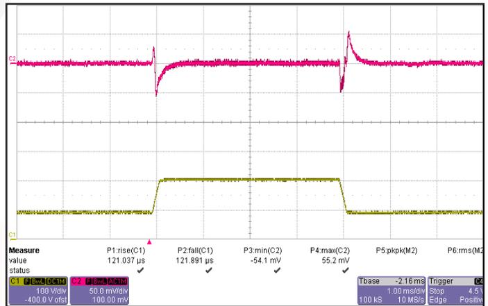
**Figure 12:** Output voltage response to step-change in input voltage (1000V/ms). Load capacitance: 10  $\mu$ F electrolytic tantalum and 1 $\mu$ F ceramic. Ch 1: Vin (100V/div), Ch 2:  $V_{out}$  (50mV/div).
