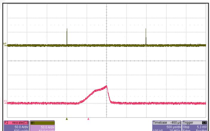
Figure 18: Load current (50A/div) as a function of time (0.5ms/div and 50ms/div) when the converter attempts to turn on into a 10 mΩ short circuit.
