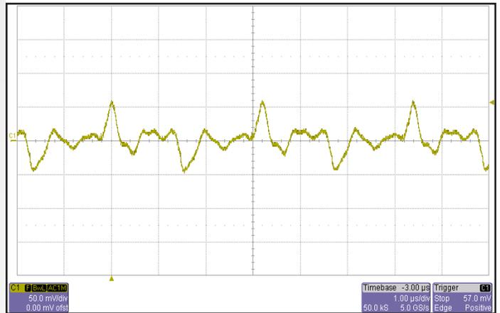
**Figure 10:** Output voltage ripple,  $V_{out}$ , at nominal input voltage and rated load current (50 mV/div). Load capacitance: 1 $\mu$ F ceramic capacitor and 10 $\mu$ F tantalum capacitor. Bandwidth: 10 MHz. See Figure 17.
