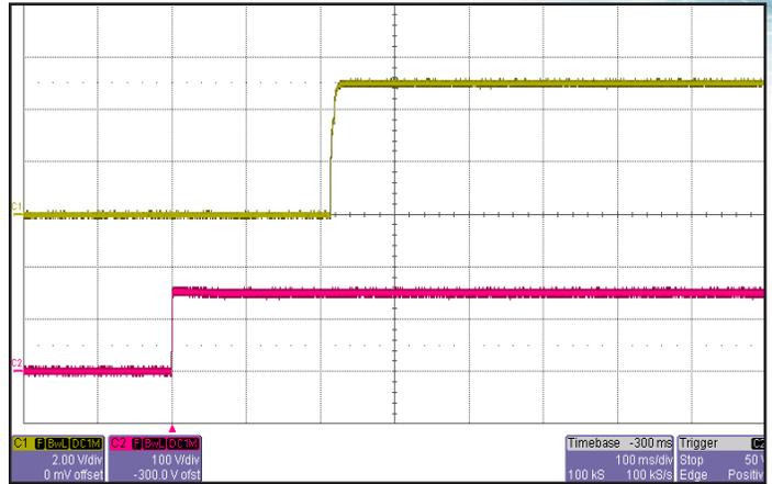
**Figure 8:** Turn-on transient at full resistive load and zero output capacitance initiated by Vin. ON/OFF Pin previously low. Ch 1: Vout (2V/div). Ch 3: Vin (100V/div).
