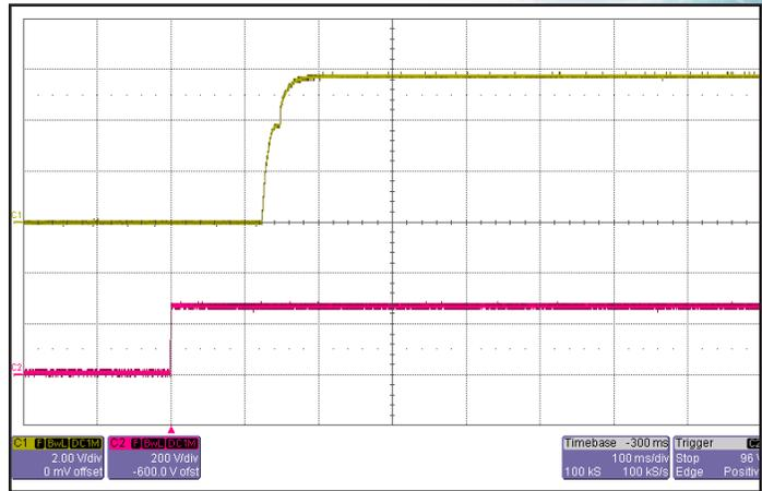
**Figure 8:** Turn-on transient at full resistive load and zero output capacitance initiated by V<sub>in</sub>. ON/OFF Pin previously low. Ch 1: V<sub>out</sub> (2V/div). Ch 2: V<sub>in</sub> (200V/div). Timescale: 100ms/div.
