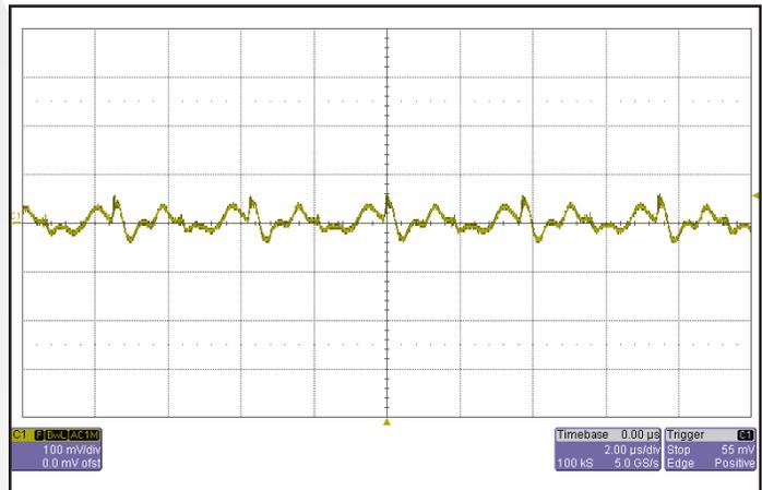
**Figure 10:** Output voltage ripple, V<sub>out</sub>, at nominal input voltage and rated load current (100 mV/div). Load capacitance: 1µF ceramic capacitor and 15µF tantalum capacitor. Bandwidth: 10 MHz. Timescale: 2.00µs/div. See Figure 17.
