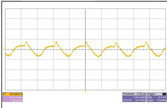
**Figure 9:** Input terminal current ripple, i<sub>C</sub>, at full rated output current and nominal input voltage with SynQor MCOTS filter module (50 mA/div). Bandwidth: 20MHz. Timescale: 1.00µs/div. See Figure 17.
