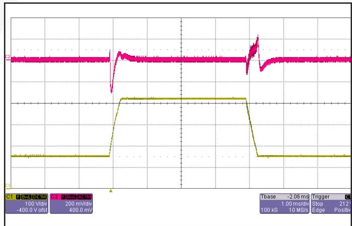
**Figure 12:** Output voltage response to step-change in input voltage (1000V/ms). Load cap: 100 µF electrolytic output capacitance. Ch 1: V<sub>in</sub> (100V/div), Ch 2: V<sub>out</sub> (200mV/div). Timescale: 1.00ms/div.
