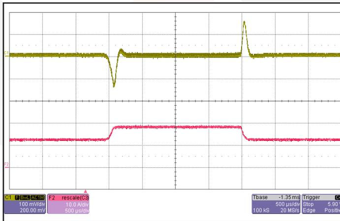
**Figure 11:** Output voltage response to step-change in load current (50%-75%-50% of I<sub>out</sub>(max); dI/dt = 0.1 A/µs). Load cap: 1 µF ceramic and 15 µF tantalum capacitors. Ch 1: V<sub>out</sub> (100mV/div), Ch 2: I<sub>out</sub> (10A/div). Timescale: 500µs/div.
