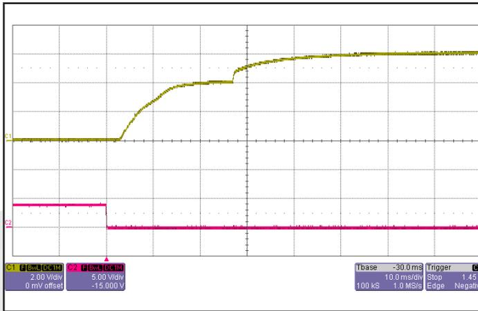
**Figure 7:** Typical startup waveform. Input voltage pre-applied, ON/OFF Pin on Ch 2. Timescale: 10.0ms/div.
