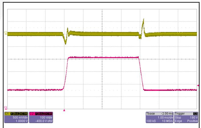
Figure 12: Output voltage response to step-change in input voltage (250V/ms). Load cap:  $1\mu F$  ceramic and  $15\mu F$  tantalum capacitors. Ch 1:  $V_{out}$  (500mV/div), Ch 2:  $V_{in}$  (100V/div). Timescale:  $1.00ms$ /div.
