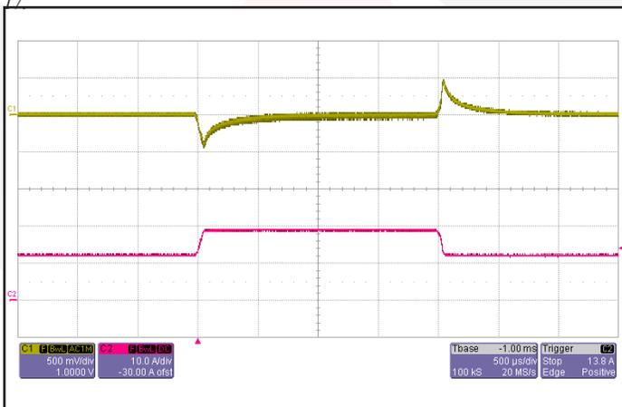
Figure 11: Output voltage response to step-change in load current (50%-75%-50% of  $I_{out(max)}$ ;  $dI/dt = 0.1 A/\mu s$ ). Load cap:  $1\mu F$  ceramic and  $15\mu F$  tantalum capacitors. Ch 1:  $V_{out}$  (500mV/div), Ch 2:  $I_{out}$  (10A/div). Timescale:  $500\mu s$ /div.
