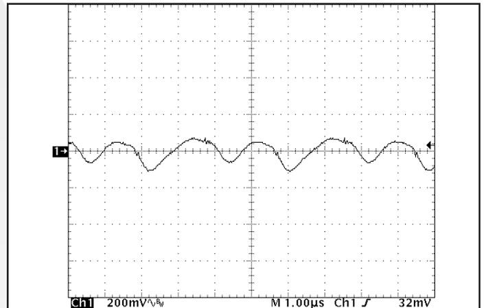
Figure 10: Output voltage ripple,  $V_{out}$ , at nominal input voltage and rated load current (200 mV/div). Load capacitance:  $1\mu F$  ceramic capacitor and  $15\mu F$  tantalum capacitor. Bandwidth: 10 MHz. Timescale:  $1.00\mu s$ /div. See Figure 17.
