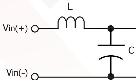
Figure E: Internal Input Filter Diagram (Component values listed on page 3)
