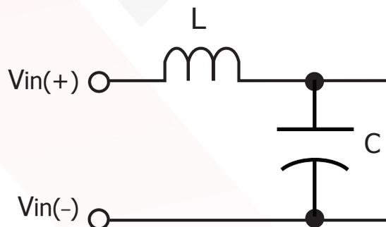
Figure E: Internal Input Filter Diagram (Component values listed on page 3)
