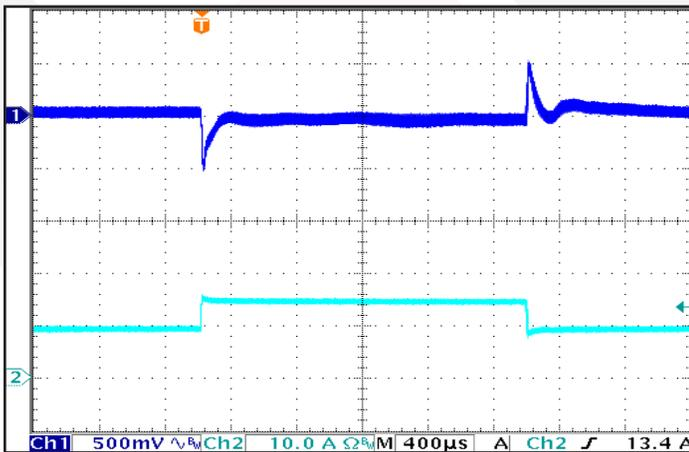
**Figure 11: Output Voltage Response to Step-Change in Load Current** (50%-75%-50% of  $I_{out(max)}$ ;  $di/dt = 5 A/\mu s$ ). Load cap: 1 uF ceramic and 100 uF electrolytic capacitors. Ch 1:  $V_{out}$  (500mV/div), Ch 2:  $I_{out}$  (10A/div), Time (400us/div).
