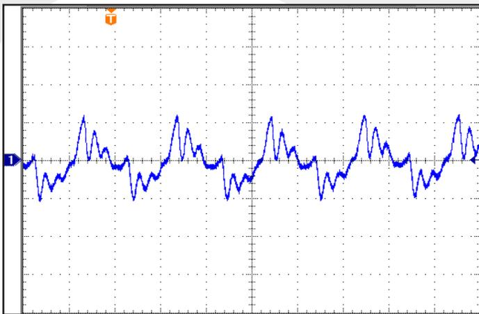
**Figure 9: Input Terminal Current Rpple**,  $i_C$  at full rated output current and nominal input voltage with 220uF electrolytic capacitor. Bandwidth: 20MHz (See Figure 13). Ch 1: Input current (1A/div), Time (2us/div).
