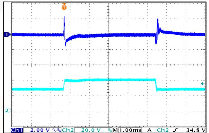
**Figure 12: Output Voltage Response to Step-Change in Input Voltage** (250V/mS). Load cap: 100 uF electrolytic output capacitance. Ch 1:  $V_{out}$  (2V/div), Ch 2:  $V_{in}$  (20V/div), Time (1mS/div).
