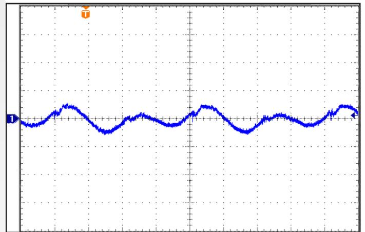
**Figure 10: Output Voltage Ripple**,  $V_{out}$ , at nominal input voltage and rated load current. Load capacitance: 1uF ceramic capacitor and 100uF electrolytic capacitor. Bandwidth: 20 MHz (See Figure 13). Ch 1:  $V_{out}$  (100mV/div), Time (2us/div).
