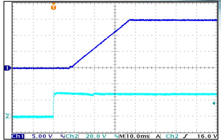
**Figure 8: Turn-on transient** at full resistive load and zero output capacitance initiated by  $V_{in}$ . ON/OFF Pin previously low. Ch 1:  $V_{out}$  (5V/div), Ch 2:  $V_{in}$  (20V/div), Time (10ms/div).
