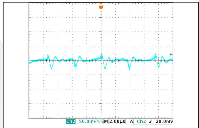
Figure 10: Output voltage ripple,  $V_{out}$ , at nominal input voltage and rated load current (50 mV/div). Load capacitance: 1µF ceramic capacitor and 10µF tantalum capacitor. Bandwidth: 10 MHz. See Figure 17.
