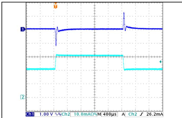
Figure 11: Output voltage response to step-change in load current (50%-75%-50% of  $I_{out(max)}$ ;  $dI/dt = 0.1 A/\mu s$ ). Load cap: 1 µF ceramic and 15 µF tantalum capacitors. Ch 1:  $V_{out}$  (1V/div), Ch 2:  $I_{out}$  (2A/div).
