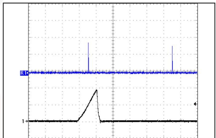
Figure 18: Load current (20A/div) as a function of time (200 $\mu s$ /div and 40ms/div) when the converter attempts to turn on into a  $10 m\Omega$  short circuit.
