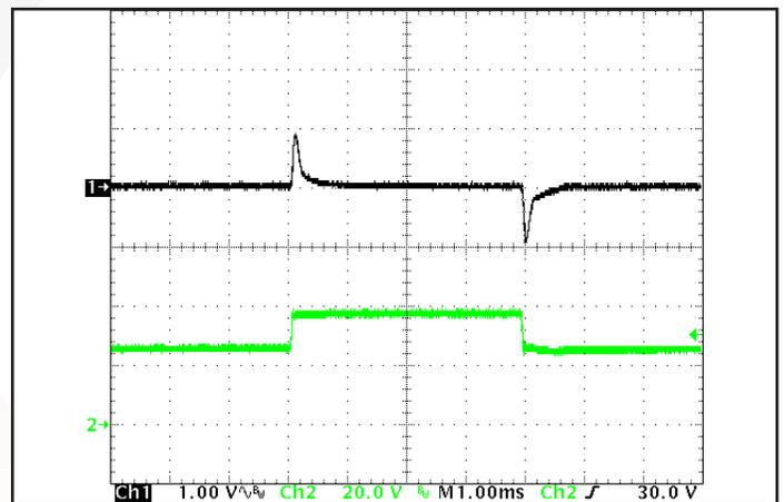
Figure 12: Output voltage response to step-change in input voltage (500V/ms) at full load current. Load cap: 100µF electrolytic capacitance. Ch1: Vout (1V/div), Ch 2: Vin (20V/div).
