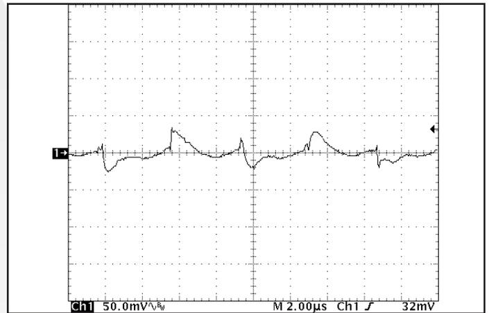
Figure 10: Output voltage ripple, Vout, at nominal input voltage and rated load current (50 mV/div). Load Capacitance: 1µs ceramic capacitor. Bandwidth: 20 MHz. See Figure 17.
