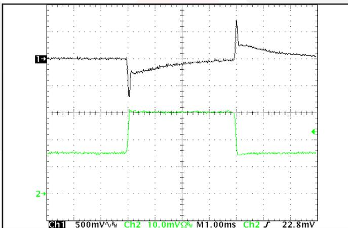
Figure 11: Output voltage response to step-change in load current (50%-75%-50% of Iout(max);  $di/dt = 0.1 \text{ A}/\mu\text{s}$ ). Load cap: 1 µF ceramic capacitor. Ch 1: Vout (500mV/div), Ch 2: Iout (5A/div).
