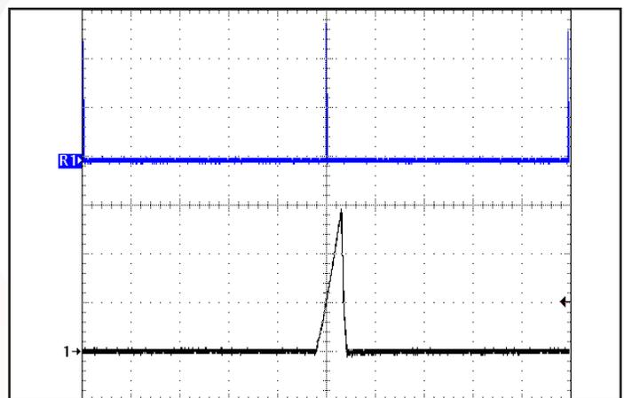
Figure 18: Load current (10A/div) as a function of time (400 $\mu$ s/div) when the converter attempts to turn on into a 10 m $\Omega$  short circuit. Reference 1 (40ms/div).
