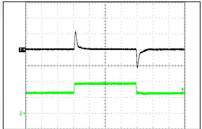
**Figure 12:** Output voltage response to step-change in input voltage at full load current. Load cap: 100 $\mu$ F electrolytic capacitance. Ch1:  $V_{out}$  (1V/div), Ch 2:  $V_{in}$  (20V/div). Time Scale (1ms/div).
