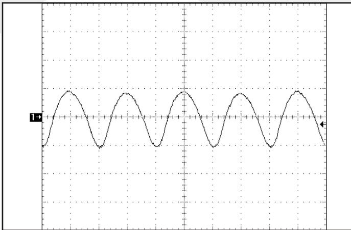
**Figure 9:** Input terminal current ripple,  $i_C$ , at full rated output current and nominal input voltage with SynQor MCOTS filter module (1 A/div). Bandwidth: 20MHz. Time Scale (2 $\mu$ s/div). See Figure 17.
