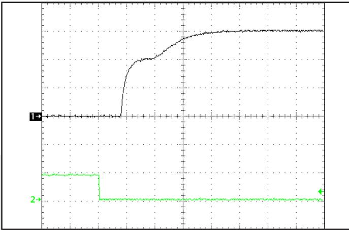
**Figure 7:** Typical startup waveform. Input voltage pre-applied, Ch 1:  $V_{out}$  (5V/div). Ch 2: ON/OFF (5V/div). Time Scale (5ms/div).
