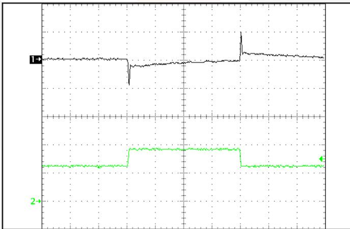
**Figure 11:** Output voltage response to step-change in load current (50%-75%-50% of  $I_{out(max)}$ ;  $dI/dt = 0.1$  A/ $\mu$ s). Load cap: 1  $\mu$ F ceramic capacitor. Ch 1:  $V_{out}$  (500mV/div), Ch 2:  $I_{out}$  (5A/div). Time Scale (1ms/div).
