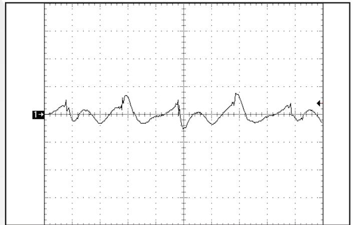
**Figure 10:** Output voltage ripple,  $V_{out}$ , at nominal input voltage and rated load current (50 mV/div). Load Capacitance: 1 $\mu$ F ceramic capacitor. Bandwidth: 20 MHz. Time Scale (2 $\mu$ s/div). See Figure 17.
