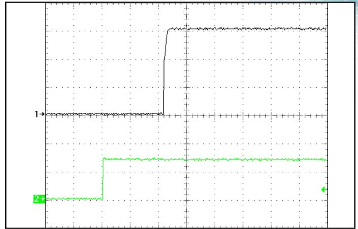
**Figure 8:** Turn-on transient at full resistive load and zero output capacitance initiated by  $V_{in}$ . ON/OFF Pin previously low. Ch 1:  $V_{out}$  (5V/div). Ch 2:  $V_{in}$  (20V/div). Time Scale (100ms/div).
