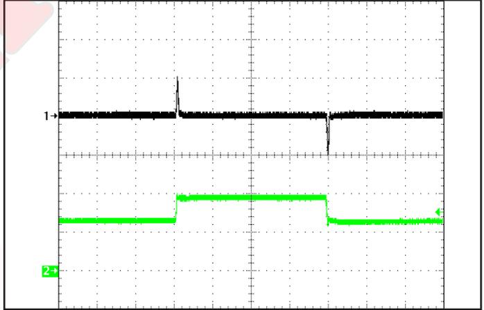
**Figure 12:** Output voltage response to step-change in input voltage (500V/ms) at full load current. Load cap: 100uf electrolytic capacitance. Ch1: Vout (.5V/div), Ch 2: Vin (20V/div).
