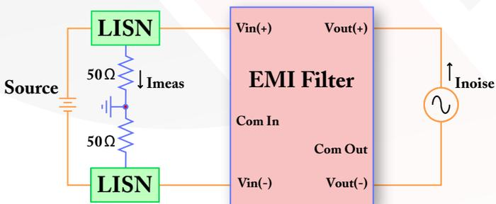
Figure B: Differential-Mode Current Attenuation,  $I_{meas} / I_{noise}$
