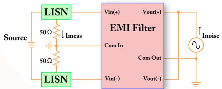
Figure C: Common-Mode Current Attenuation,  $I_{meas} / I_{noise}$
