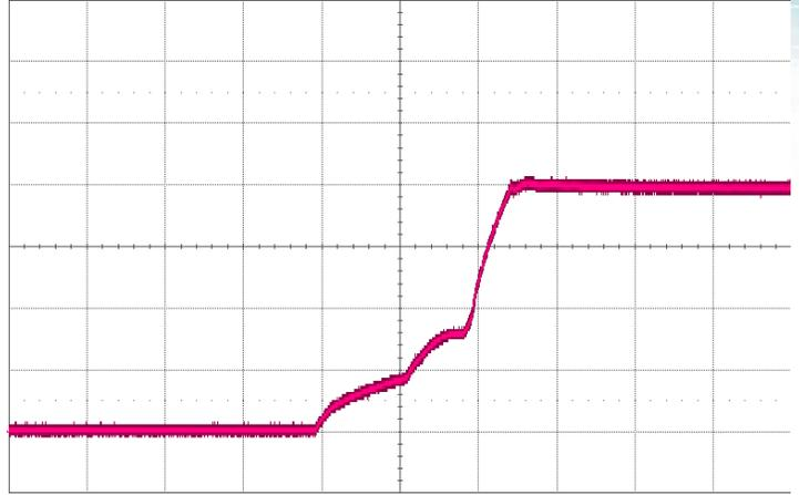
Figure 8: Output voltage startup waveform with 200 $\mu$ F hold-up capacitor, no load (115VAC, 60Hz) Vout (100V/div), Timebase: (500ms/div)
