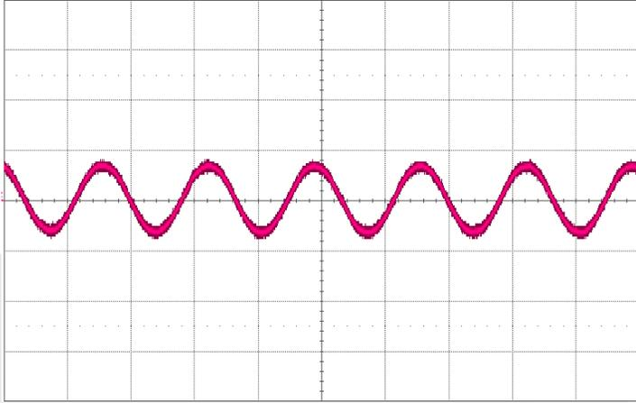
Figure 7: Output voltage ripple with 200 $\mu$ F Hold-up capacitor at full rated power (115VAC, 60Hz) Vout (10V/div), Timebase: (5ms/div)
