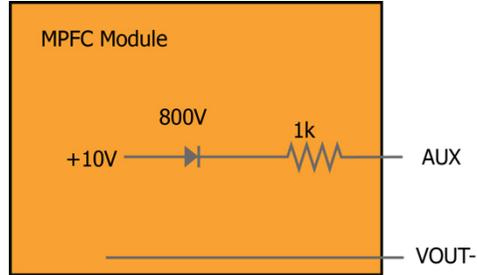
The purpose of the AUX power supply is to provide a low level of power to control circuitry at the output of the MPFCQor, such as the circuits shown earlier in this section.
