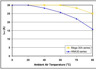
Figure 5: Comparison of Power Derating curves for Mega Figure 6: Comparison of Power Derating curves for Giga series versus the original HNA 30 series for 3.3Vout modules at series versus the original HNA 40 series for 3.3Vout modules at nominal 48Vin and 200 LFM of airflow.
