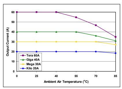
**Figure 2**: Power derating curves at 300 LFM airflow for the Kilo, Mega, Giga, and Tera versions of the 48Vin, 2.5Vout PowerQor dc/dc converters.
