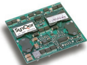
Figure 3: SynQor converter with no heatsink or baseplate
