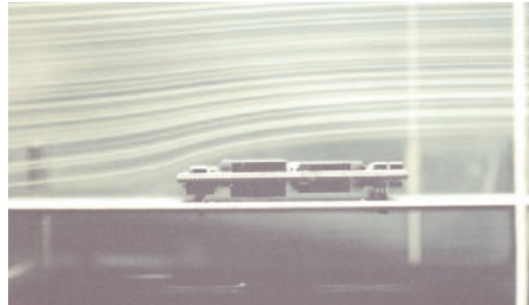
Figure 9b: Airflow over SynQor converter showing small boundary layer
